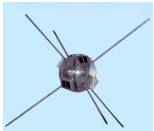
Vanguard I, 1958 – First Solar powered satellite.
